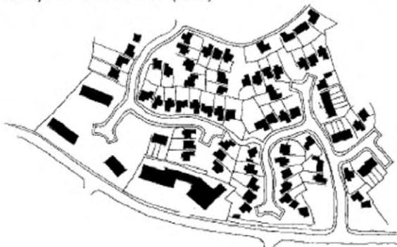
Cul-de-sac design that increases segregation and reduces interaction of communities and surroundings should be avoided
