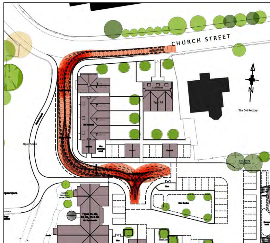
Above: Vehicle tracking demonstrating access and turning within the site is capable by a large refuse collection vehicle (Drawing courtesy of Caunton Properties Ltd, highway consultants Stirling Maynard and JWA Architects).
