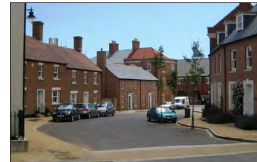
Informal on-street parking provided by subtle widening of the carriageway
