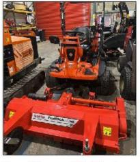
Front Mounted Flail Deck An out-front powerful flail mower. This machine makes quick work in even the toughest terrain.
